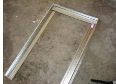
You can create a filter tray out of bent sheet metal or drip edge flashing.
