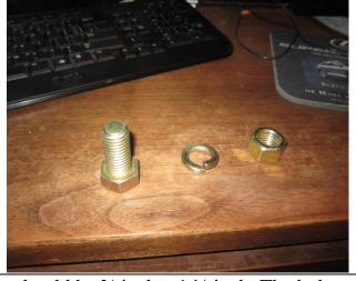
The bolts securing the angle iron to the I-Beam should be ¾ inch x 1 ½ inch. The bolts, locking washers and nuts should be Grade 8. Grade 8 bolts are stronger than commonly used Grade 5 bolts and provide higher tensile strength.
