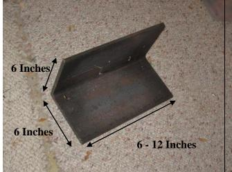
To stabilize a main steel beam we recommend using 3/8 inch angle iron at 6 inch x 6 inch. The length should be around 6-12 inches.
